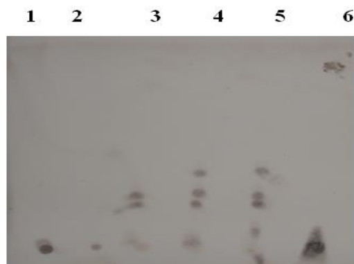
Fig. 9: TLC using silica gel showing pattern of product formation by action of Endo-PGase on polygalacturonic acid at 55°C after different incubation time: Lane 1: control-1, only polygalacturonic acid; Lane 2: 0 min; Lane 3: 10 min; Lane 4: 20 min; Lane 5: 40 min; Lane 6: control-2, only galacturonic acid.
